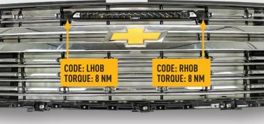
**INSTALLATION PROCESS** - Linear-18 shown for illustration purposes. Install should be completed with the grille left on the vehicle.
