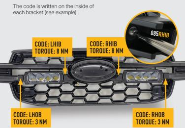
**INSTALLATION PROCESS** - Install should be completed with the grille left on the vehicle.
