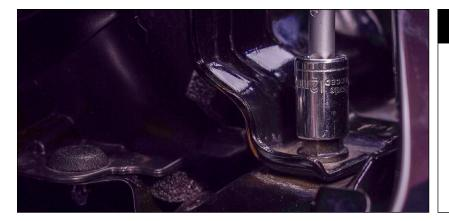
Once the stud is installed, remove the front hinge bolt.
