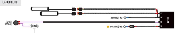
Customer's have the option to connect to a positive battery or ignition feed. Connecting to the ignition feed, the light will only operate with the ignition turned on.
