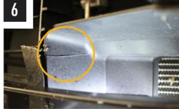
The Air Dam will need to be cut horizontally slightly to allow flexability for the Air Dam to sit under the lamp (complete step on both sides).
