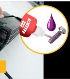
Please use a thread seal compound (i.e. Loctite 222) to protect the lamp fastener from binding over time.
