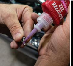
Insert the lamps into the mounting bezel and secure the lamps using the supplied lamp fixtures (Torque values and bolt sizes adjacent). Please use a thread seal compound (i.e. Loctite 222) to protect the lamp fastener from binding over time.
