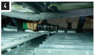
Remove 3x 10mm bolts holding the Active air shutter to the grille. (Removing the other 3x10mm bolts at the bottom of the active air shutters will give you more room to work but is not necessary)
