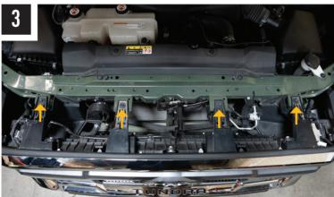
Remove 4x 10mm bolts holding grille to radiator support
